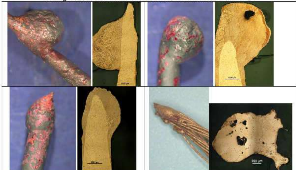
Figure 6 Stereomicroscope and optical micrographs of fire melting damage to solid and stranded conductors created in the laboratory.
